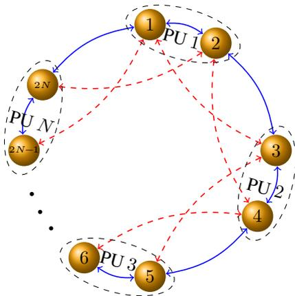
Figure 1. Closed chain of  $N$  identical PU oscillators.
