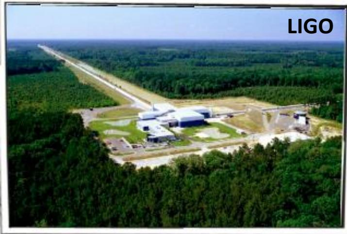
$$h \sim \frac{\Delta L}{L} \sim \frac{10^{-18} \text{ m}}{4 \text{ km}}$$
