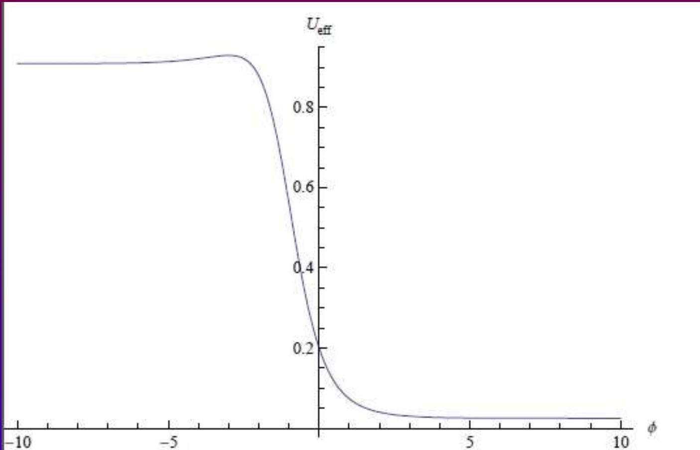
Qualitative shape of the effective scalar potential  $U_{\text{eff}}$  (14) as function of  $\varphi$  for  $M_1 < 0$ .
