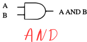
Fig. 2.3 The AND Gate
